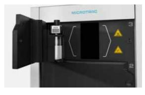
The measurement cell is placed directly in the trap door's sample holder.
