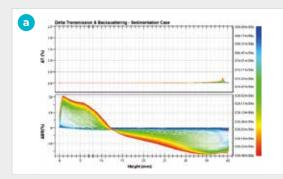
Transmission and backscattering in function of the sample height
